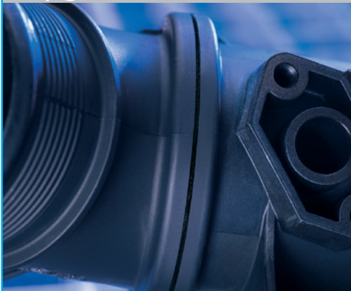
Vibration weld seam
