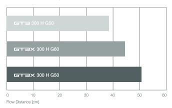
Product comparison TEREZ® GT3/GT3X Flow-spiral with 2 mm wall thickness
